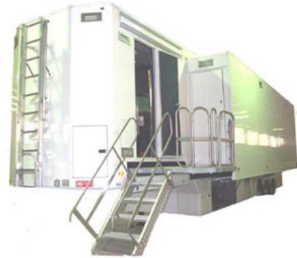
Front view with entrances into the Audio and Video sections. A Front ladder provides access to the roof stand area.
